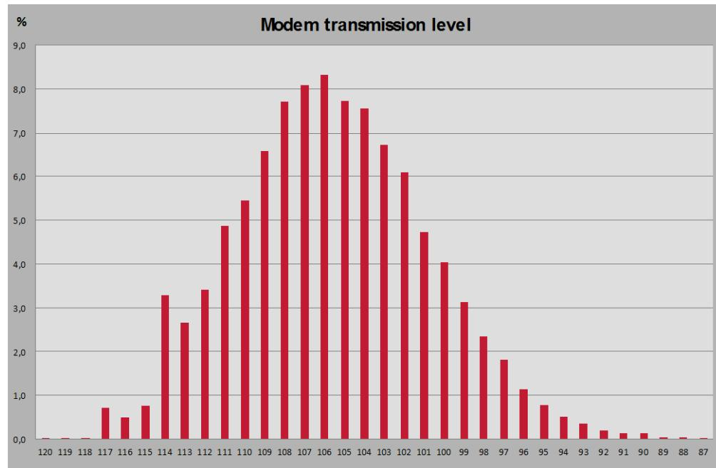
The large spread in the return path attenuation results in a large spread in transmission level from each modem as the CMTS controls the modem so the received signal level is equal from all modems.
